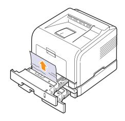
Insert the trays back into the printer. Printing automatically resumes.
